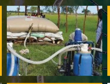
Water treatment system contains water storage, Pipes, Water Treatment Unit and bladder for water distribution.
